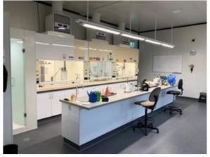
Figure 4: ALCORE test lab, fume cabinets with hi-tech scrubbers, showers, microscopes & Draegar air monitor (wall)
