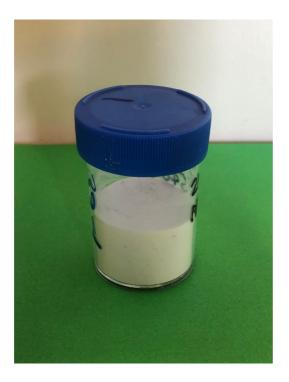
Figure 1: Alcore AIF<sub>3</sub> sample produced from combination of dross and aluminium hydroxide.
