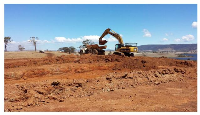
Figure 4: Mining, loading & hauling bauxite ore at Bald Hill Bauxite Project.
