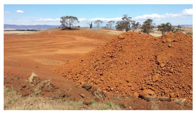
Figure 6: Stockpiled bauxite at the screening site. Screening plant arrived at site 29 January to commence screening trials on 30 January. A second bauxite pit workings is in the distance (top centre). Because this second pit is high grade, it will be screened once the screening process has been optimised.
