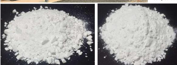
Figure 10: Commercial-grade and well-crystallised AIF<sub>3</sub> samples made at the Alcore Research Centre in June
