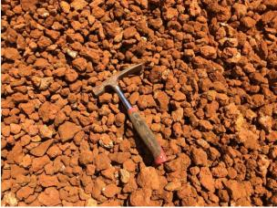
Figure 9 Cement-grade bauxite product
