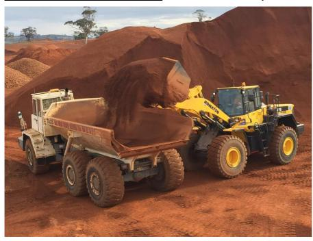
Figure 5 Blending cement-grade bauxite at Bald Hill Mine Site
