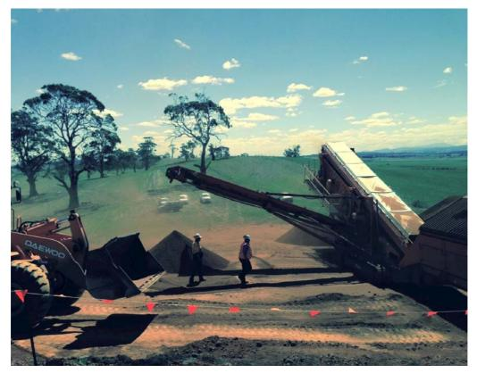
Figure 3: Sampling screened bauxite products at Bald Hill Bauxite Project, Tasmania
