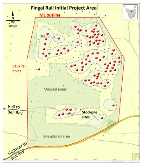
Figure 18 Fingal Rail Bauxite Project Drillholes: red holes
