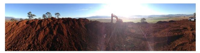
Figure 5: Each run-of-mine bauxite stockpile is from a single bench from a specified pit for product management
