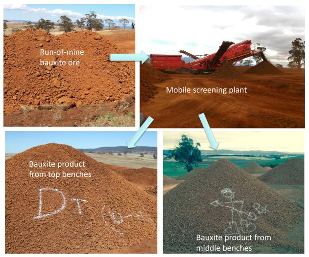
Figure 10: Processing flowsheet at Bald Hill Bauxite Project. Stockpile labelling codes are being simplified.
