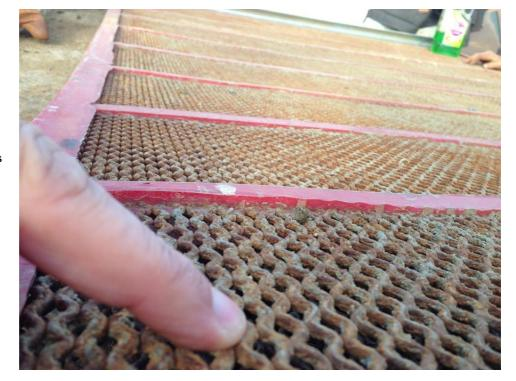
Figure 9: Polyvibe 7mm aperture screens are being used as the bottom screen size to optimise grades and yields.
