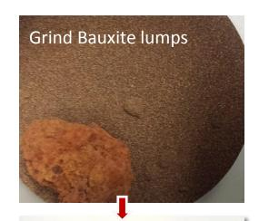
**Bauxite** =  $36\% \text{ Al}_2\text{O}_3$   $25\% \text{ Fe}_2\text{O}_3$   $10\% \text{ SiO}_2$   $5\% \text{ TiO}_2$  &  $23\% \text{ H}_2\text{O}$  **Reagents** are mixtures of:
