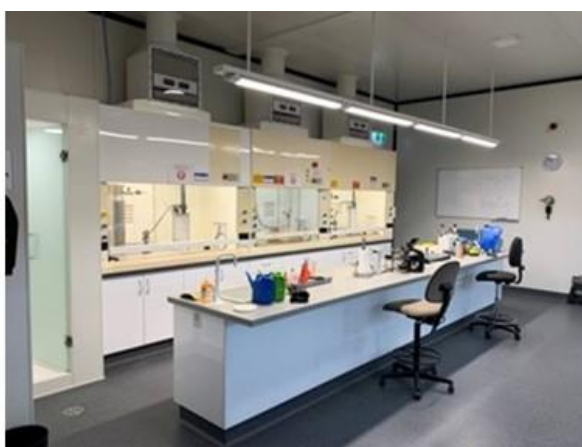
Figure 5: Alcore test lab, fume cabinets with hi-tech scrubbers, showers, microscopes & Dräger air monitor (wall)
