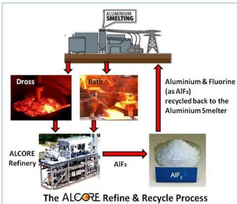
Figure 3 Summary of the Alcore 'Refine & Recycle' strategy This process has the strong potential to be the simplest and lowest cost method to make AlF_3 . It provides an economically attractive way to utilise the aluminium-rich and fluoride-rich by-products from many aluminium smelters.
