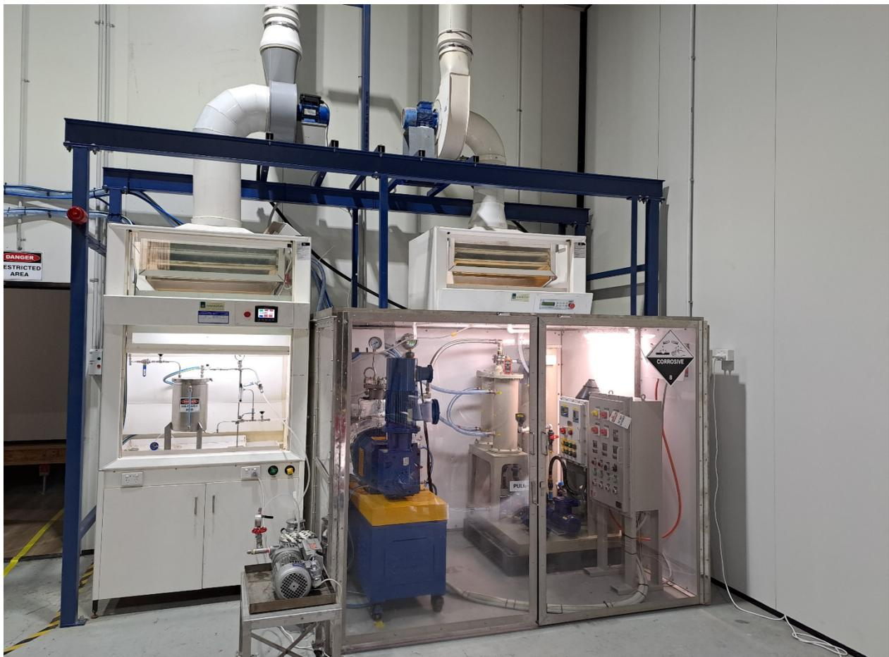
**Figure 1: Bath pilot batch reactor (centre) fully commissioned with operations underway**
