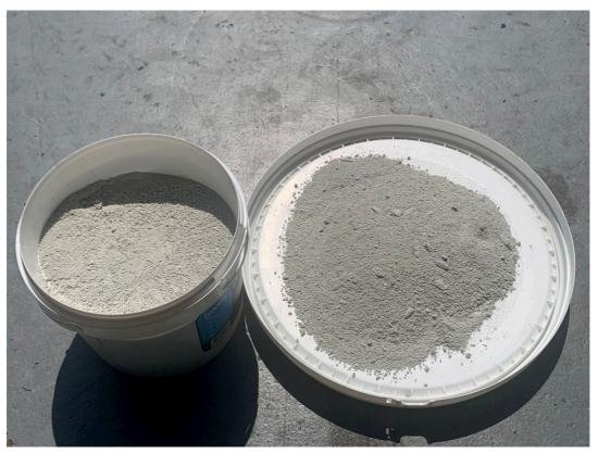
Figure 2: Sample of metal sulfate powder produced from bath pilot batch reactor.
