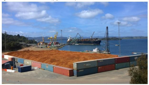
Figure 2: The 30,000 tonne cargo assembled at Bell Bay export ports. Note that the containers are used as dust barriers to prevent cross contamination with other cargoes. The bauxite is shipped in bulk carrier ships similar to the ship shown here.
