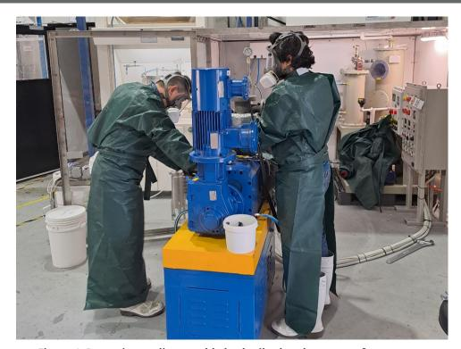
Figure 1: Preparing to disassemble bath pilot batch reactor after test run
