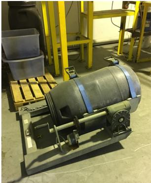
Pre-existing forklift mounted electric drum rotator for safe, remote discharge of bauxite into the ore hopper
