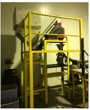
Pre-existing ore hopper & screw feed to granulators & sieve.
