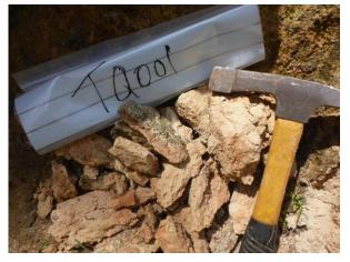
Figure 4: Sample TQ001 refractory bauxite, bottom layer
