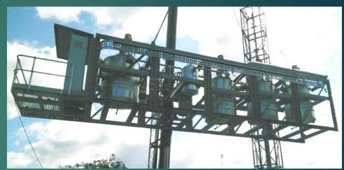
Typical skid mounted processing unit produced by Turnkey Innovative Engineering
