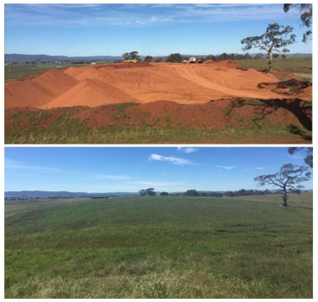
Figures 19 & 20: Pits MB5 & 6 during mining and after rehabilitation Land can be restored to productive standard within 2 or 3 years – as shown for the rehabilitated mined area above.
