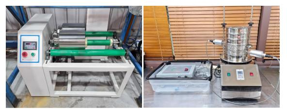
Figure 1: Ball mill (left) and ultrasonic vibrating screen (right), which enable ALCORE to prepare bath with a narrower range of particle sizes.
