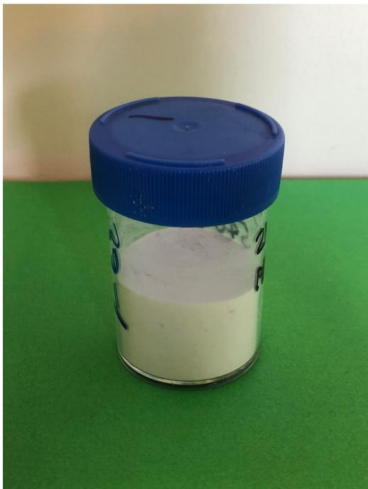
Figure 1: Alcore  $\text{AlF}_3$  sample produced from combination of dross and aluminium hydroxide.
