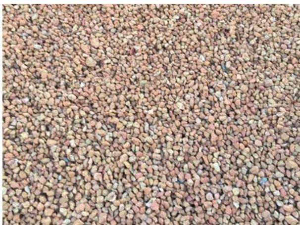
Figure 8: Close-up of the stockpiled bauxite
