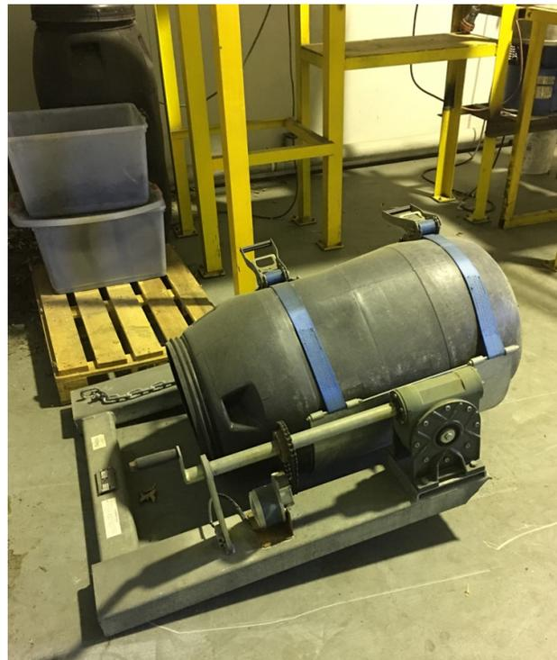
Pre-existing forklift mounted electric drum rotator for safe, remote discharge of bauxite into the ore hopper
