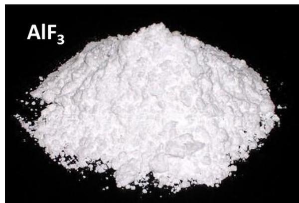
Figures 1, 2 & 3: AlF<sub>3</sub> is added daily into aluminium smelter potlines to maintain efficiency. There is no substitute.
