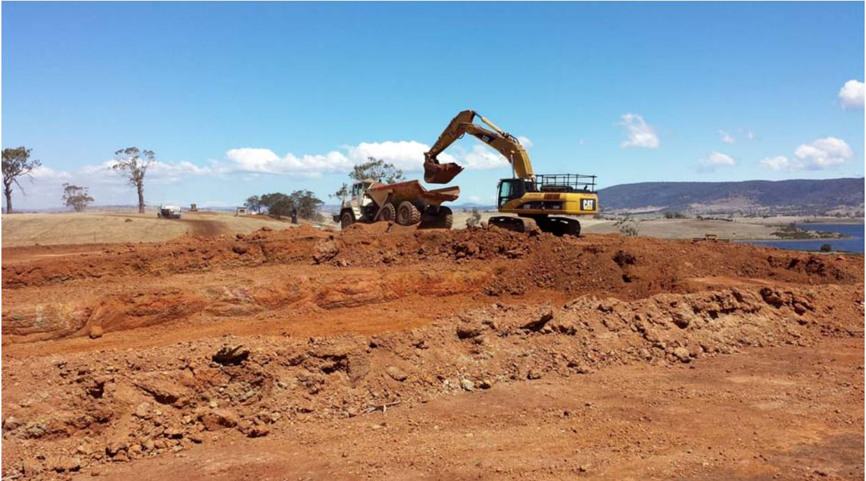
**Figure 4: Mining, loading & hauling bauxite ore at Bald Hill Bauxite Project.**
