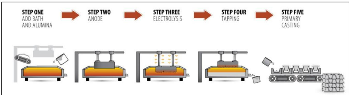
Figure 19: Aluminium smelting (Source: Australian Aluminium Council)
