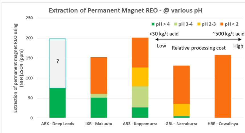
Figure 13: Extraction rates and required pH for extraction (Source: ASX announcements, CC & ABx)
