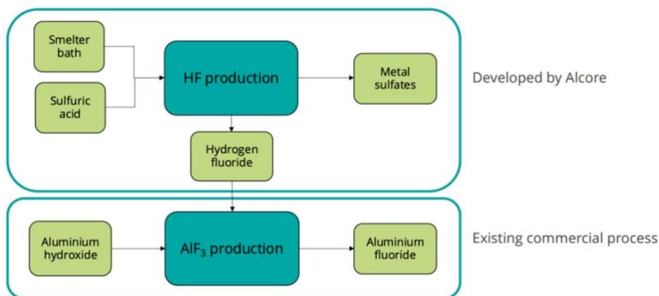
Figure 18: Alcore Simplified Flow sheet (Source: ABx)
