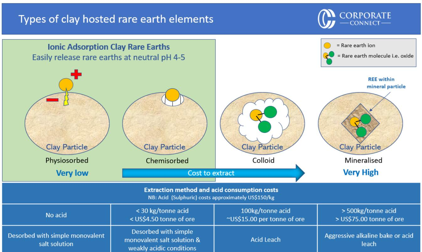
Figure 11: Types of Clay hosted REE deposits - and the cost of extraction (Source: Corporate Connect)
