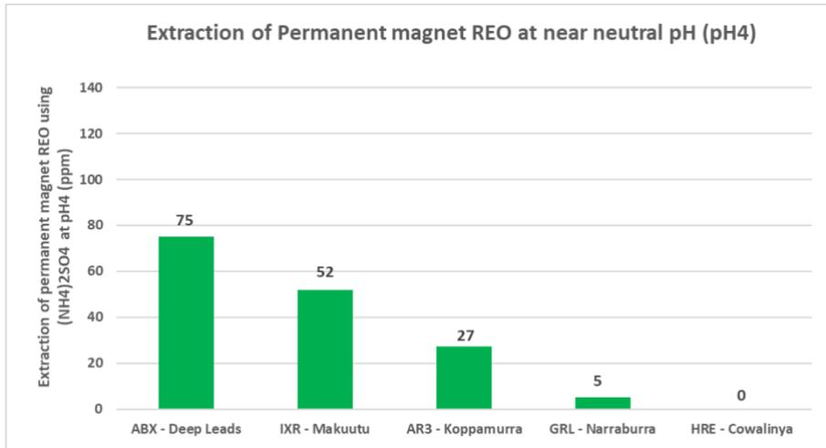
Finally, Figure 14 demonstrates the level of Permanent Magnet extraction that is achievable under the lowest cost regime of pH4 and weak Ammonium Sulphide solution.
