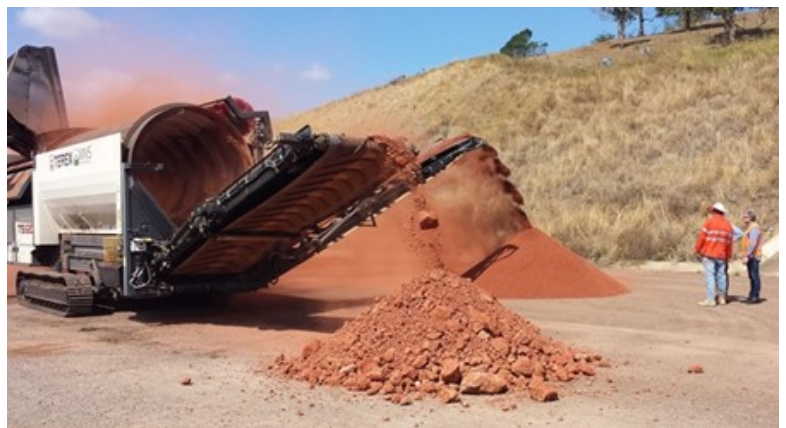
Figure 2: Screening of 28 tonnes of Binjour bauxite at Gympie
